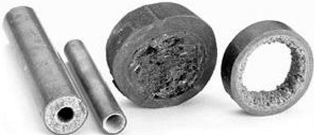
Fig. 1 Photograph of fouled heat-exchanger tube.
